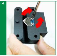
Remove the two screws that secure the worn blade using the Phillips screwdriver (4). WARNING! The blade has two
