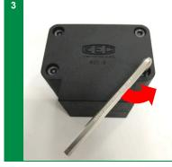
To replace the blade, proceed by unscrewing the four TCEI screws with the Allen wrench (3) and separate the two halves that make up the Splitting Tool (2).
