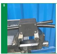
Continue to insert the twin hose into the Splitting Tool (2) until the desired separation length is achieved. Visually check the good result of the operation.
