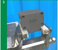
Lock tight the Splitting tool (2) on a bench vise as shown in the figure beside.
