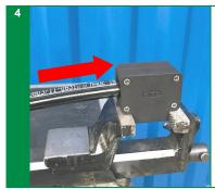
Insert the twin hose either on one side or the other of the Splitting Tool (2). Exert a slight force to overcome the initial resistance to cutting.
